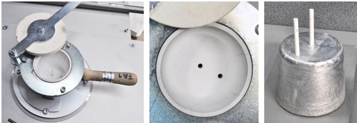
Figure 3. Thermal analysis ceramic cup and samples with two thermocouples.
